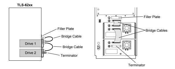
Figure 4-1 TLS-62xx and 82xx Drive Cabling Diagram
